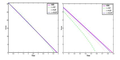
Figure 1: Left: computed values of area A(t) by (28), and by a modified ETD4 scheme for (27) using  $\epsilon = 0.5, 0.25$  and 0.125. The picture on the right is a zoomed-in part of the left figure.
