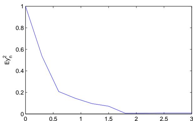
Fig. 5.2. Mean square stability of SST method with  $\theta = 0.6$  and  $\Delta t = 0.6$
