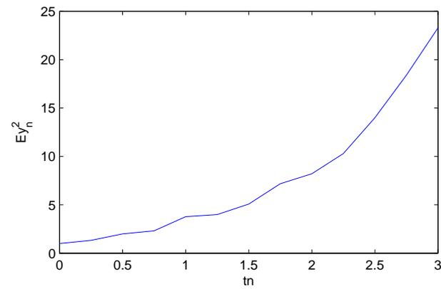
Fig. 5.6. Unstable test for SST method with  $\theta = 0.1$  and  $\Delta t = 0.8$
