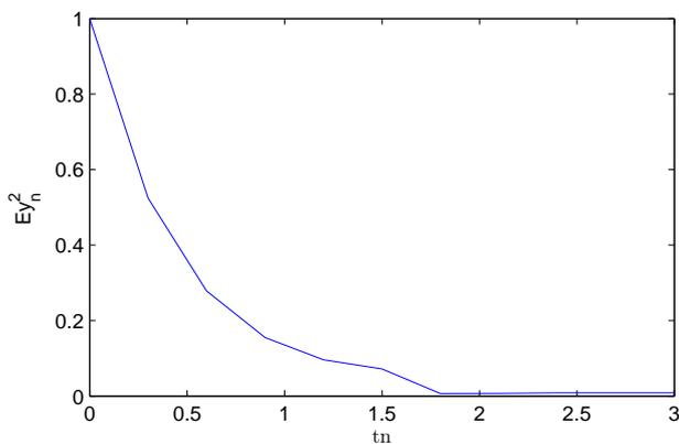
Fig. 5.1. Mean square stability of SST method with  $\theta = 0.6$  and  $\Delta t = 0.1$
