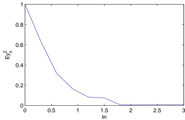
Fig. 5.5. Mean square stability of SST method with  $\theta = 0.1$  and  $\Delta t = 0.6$
