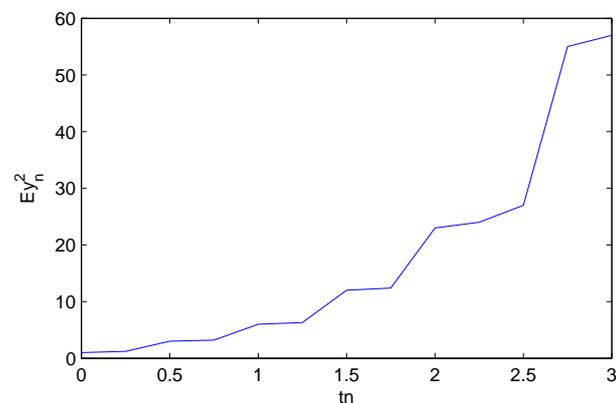
Fig. 5.3. Unstable test for SST method with  $\theta = 0.6$  and  $\Delta t = 0.8$
