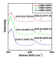
Figure 6: The SERS spectra of 2-MBA (red line), 3-MBA (green line) and 4-MBA (blue line) from 1500 to  $2500 \text{ cm}^{-1}$ , with detailed intensity marked respectively.
