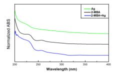
Figure 2: Absorption spectra of Ag sol (green line), 2-MBA (black line) and 2-MBA with Ag sol (blue line) from 200 to 400 nm.
