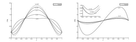
Figure 9: The time evolution of F'/Re and G/Re for the second solution under Re = -9,  $\alpha = 2$ .
