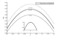
Figure 3: The time evolution of the axial velocity F'/Re for Re = 5,  $\alpha = 0$ .
