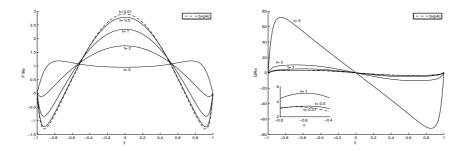
Figure 16: The time evolution of F'/Re and G/Re for the second solution under Re = -30,  $\alpha = 1.5$ .
