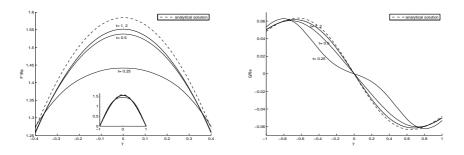
Figure 13: The time evolution of F'/Re and G/Re for Re = 5,  $\alpha = 1$ .
