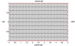
Figure 2: A triangular mesh of the rectangular channel domain  $\Omega$ .
