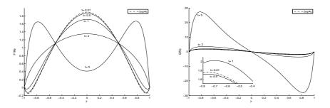
Figure 10: The time evolution of F'/Re and G/Re for the first solution under Re = -20,  $\alpha = 1$ .
