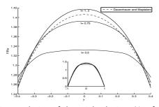
Figure 4: The time evolution of the axial velocity F'/Re for Re = 20,  $\alpha = -5$ .
