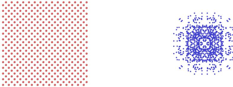
Figure 6: Configuration of atoms in stress calculation. Left: planform of perfect BCC crystal. Right: planform of virtual atoms.
