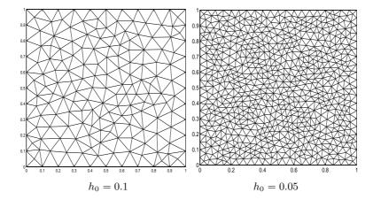
FIGURE 6. The initial meshes for the square domain
