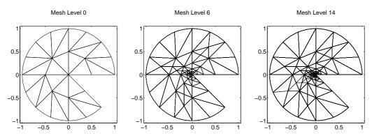
Figure 4: Example 2: The initial mesh (left) and the meshes after 6 (middle) and 14 (right) adaptive refinement steps (k = 4 and  $\Theta = 0.1$ ).
