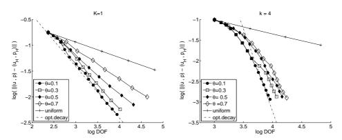
Figure 5: Example 2: The error  $||(\mathbf{u},\mathbf{p}) - (\mathbf{u}_H,\mathbf{p}_H)||$  versus the number of degrees of freedom on a logarithmic scale for various  $\theta$ , k = 1 (left) and k = 4 (right).
