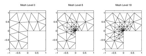
Figure 2: Example 1: The initial mesh (left) and the meshes after 8 (middle) and 18 (right) adaptive refinement steps (k = 4 and  $\Theta = 0.1$ ).
