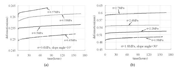
Figure 3: The grading curves of shear creep of  $10^\circ$  and  $30^\circ$  structural planes.
