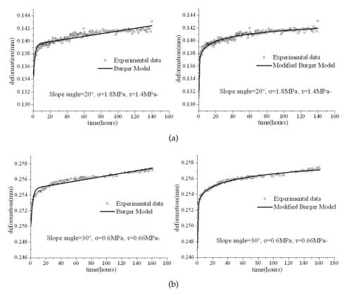
Figure 8: The test curves fitting graph of the modified Burger model and Burger model.
