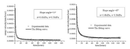
Figure 5: The fitting curves of creep velocity of structural planes.
