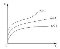
Figure 7: Creep curves of modified Burger model.
