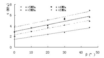
Figure 1: The relationship between peak shear strength and discontinuity angle.
