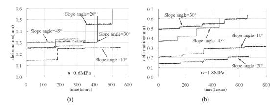
Figure 2: The curves of shear creep test process of structural planes with different slope angles.
