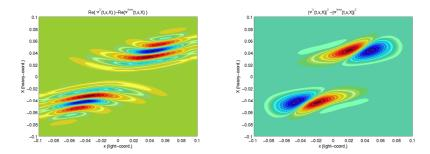
Figure 10: Dephasing effect. Left: Plot of the difference  $\mathcal{R}e(\psi(t,x,X)) - \mathcal{R}e(\psi^{\mathrm{free}}(t,x,X))$  for  $t \in [0,T_{int}]$ . Right: Plot of the difference  $|\psi(t,x,X)|^2 - |\psi^{\mathrm{free}}(t,x,X)|^2$  for  $t \in [0,T_{int}]$ .
