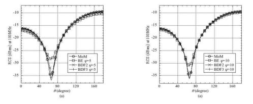
Figure 3: The RCS with oversampling factor  $\psi = 5$  and  $\psi = 10$  for the sphere as a function of elevation angle.
