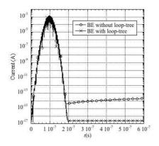
Figure 1: The average surface current computed by  $\mathsf{EFIE}$  with/without the stabilization.
