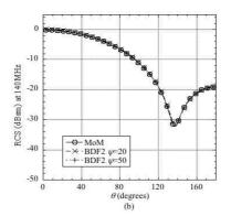
Figure 5: The RCS for dielectric cube by MoM and CQ using BDF2 (with two different oversampling factors).
