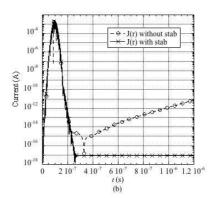
Figure 6: The surface current computed by EFIE using CQ with BDF2 for the cube scatterer with oversampling factor  $\psi = 10$ . Results with and without stabilization are shown.
