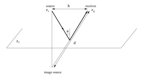
Figure 3: The main contribution in the saddle point approximation for the scattered field for the  $c_0 > c_1$  and pre-critical  $c_0 < c_1$  cases. In this picture *h* represents the horizontal offset and *d* represents the total distance traveled by the wave from source to interface to receiver.
