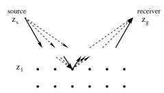
(b) Scattering diagrams of main contributions to the expression of the refracted scattered field (headwave) for a point source and a point receiver located at post-critical offset.
