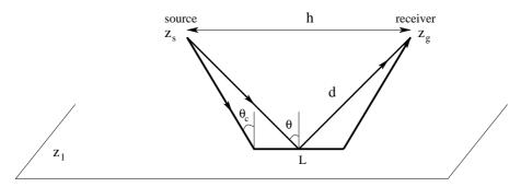
Figure 4: The main contribution in the saddle point approximation for the scattered field for the post-critical  $c_0 < c_1$  case. In this picture h represents the horizontal offset, d represents the total distance traveled by the reflected wave from source to interface to receiver and L is the horizontal part (along the interface) in the path of the headwave.
