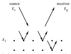
(a) Diagrammatic representation of main plane wave component contribution to the expression of the scattered field for a point source and a point receiver located at precritical offset.
