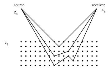
Figure 5: Diagrammatic representation of the point-scatterer interactions described by the forward scattering series. 1-, 2- and 3-interactions are shown with propagations from the source to the scatterers, between scatterers and from the scatterers to the receiver in the reference medium only.
