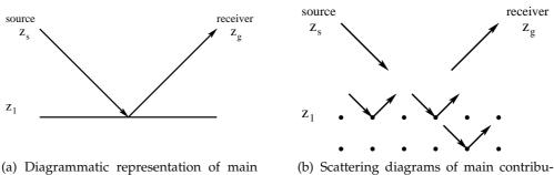
plane wave component contribution to the expression of the reflected scattered field for a point source and a point receiver located at post-critical offset.
