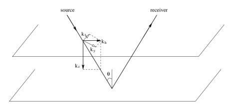
Figure 1: Horizontal and vertical wavenumbers associated with one plane wave component and satisfying the dispersion relation  $k_x^2 + k_y^2 + \nu_0^2 = \omega^2 / c_0^2$ . The picture also shows the total horizontal wavenumber,  $k_h$ , defined through the relation  $k_x^2 + k_y^2 = k_h^2$ .
