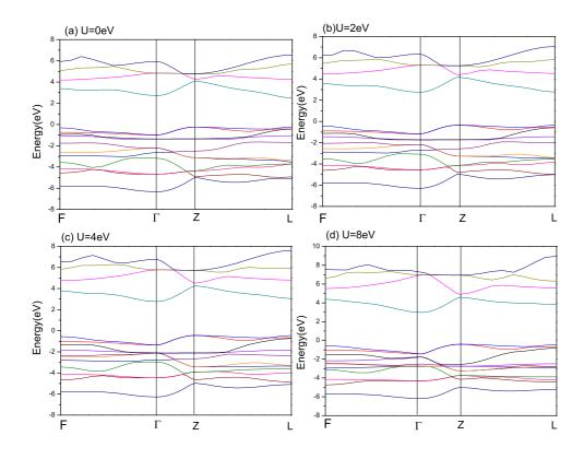
Figure 3: The band structure of CuYO<sub>2</sub> under GGA+U calculation, (a)-(d) shows the band structure under U=0, 2, 4, and 8 eV, respectively. Energy zero is set to  $E_{\rm VBM}$ .
