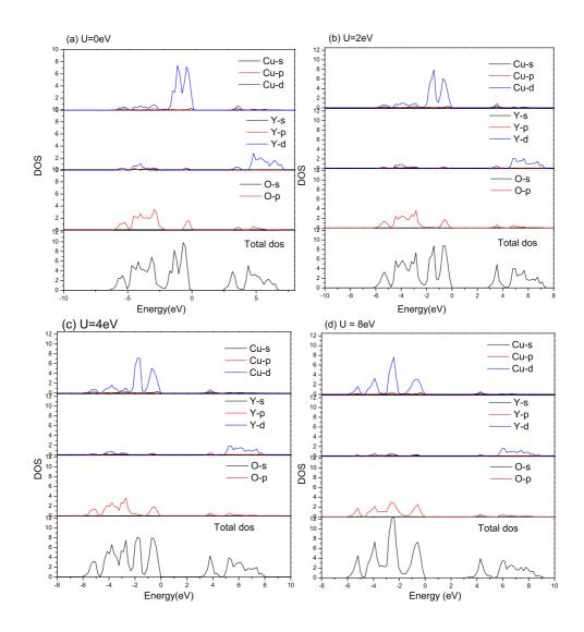
Figure 2: The total density of states and partial density of states in CuYO<sub>2</sub> under GGA+U calculation, (a)-(d) shows the density of states under U =0, 2, 4, and 8 eV, respectively. Energy zero is set to  $E_{VBM}$ .
