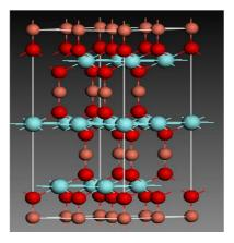
Figure 1: Crystal structures of  $CuYO_2$ , red atoms are O atoms, brown atoms are Cu atoms, blue atoms are Y atoms.
