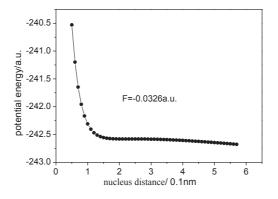
Figure 3: Potential energy curves under critical dissociation fields.
