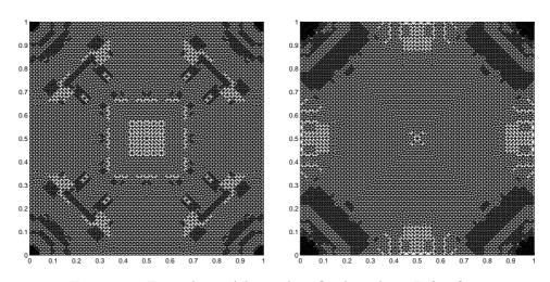
FIGURE 4. Example 1: Adaptively refined meshes. Left:  $\beta_1 = \beta_2 = \beta_3 = \beta_4 = 0.5$  (10 refinement steps, 17760 elements). Right:  $\beta_1 = \beta_2 = \beta_3 = \beta_4 = 0.99$  (10 refinement steps, 19744 elements).
