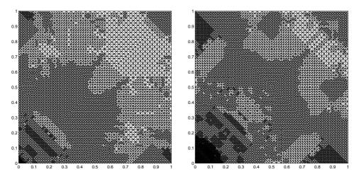
FIGURE 3. Example 1: Adaptively refined meshes. Left:  $\beta_1 = 0.5$ ,  $\beta_2 = \beta_3 = \beta_4 = 0.0$  (12 refinement steps, 11768 elements). Right:  $\beta_1 = 0.99$ ,  $\beta_2 = \beta_3 = \beta_4 = 0.0$  (13 refinement steps, 16362 elements).
