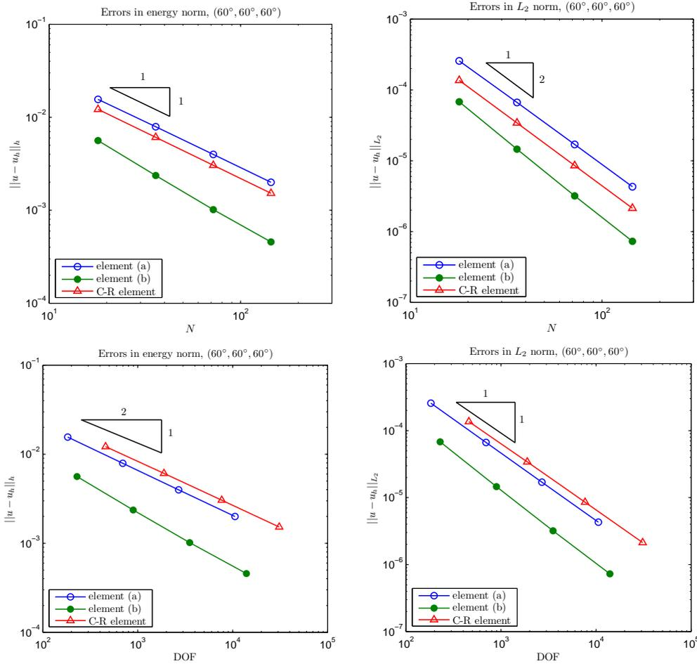
Fig. 4.3. Comparisons among the  $Q_1$  hexagonal element (element (a)), the modified  $Q_1$  hexagonal element (element (b)), and the Crouzeix-Raviart triangular element (C-R element).
