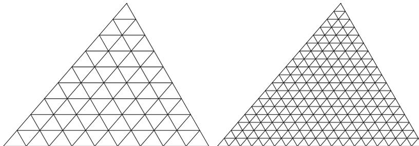
Fig. 4.2. The triangular meshes for the triangular domain  $\Omega$  (left:  $N = 9$ , right:  $N = 18$ ).
