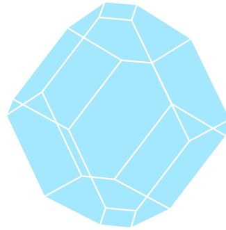
Figure 1: The Brillouin zone for a body-centered tetragonal lattice. The Brillouin zone is the integration domain of integrals that give properties of materials. It is also a convex polygon that often has a complicated shape. This plot, and many others in this article, were created with SymmetryReduceBZ (see https://github.com/jerjorg/SymmetryReduceBZ.jl ).
