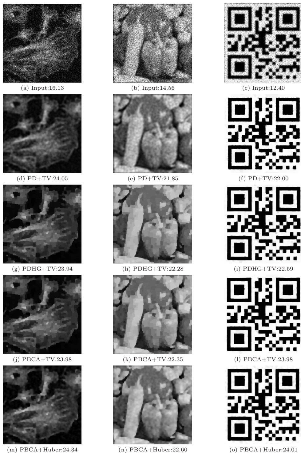
Fig. 4.7. Results of different algorithms (with PSNR(dB) below the figures) for mixed Poisson-Gaussian noise deblurring. (a): “Fluorescent Cells”, noise level: \eta = 16, \sigma = 10^{-1}, H = \text{fspecial}(\backslash\text{disk}, " 3) ; (b): “Peppers”, noise level: \eta = 16, \sigma = 10^{-2}, H = \text{fspecial}(\backslash\text{Gaussian}, " [7,7], 3) ; (c): “Two Code”, noise level: \eta = 16, \sigma = 10^{-2}, H = \text{fspecial}(\backslash\text{disk}, " 3) .
