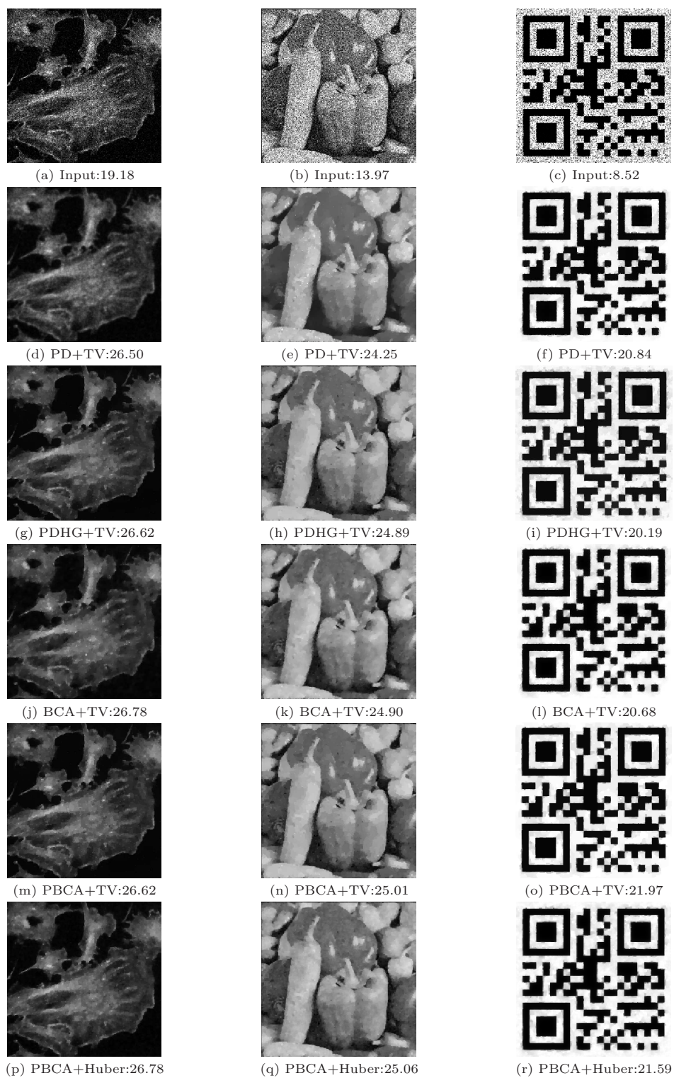
Fig. 4.10. Results of different algorithms (with PSNR(dB) below the figures) for mixed Poisson-Gaussian noise denoising. (a): “Fluorescent Cells”, noise level: \eta = 16, \sigma = 10^{-2} ; (b): “Peppers”, noise level: \eta = 16, \sigma = 10^{-1} ; (c): “Two Code”, noise level: \eta = 4, \sigma = 10^{-2} .
