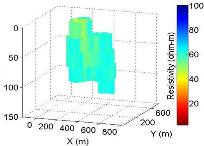
Figure 2: LQL inversion results. The resistivity values greater than 60 ohm-m are removed from the view. The locations of the bodies are evident, but the resistivity is overestimated. Note also that the lateral extents of this figure are greater than that of the figure showing the true bodies. This reflects padding at the edges of the inversion domain.
