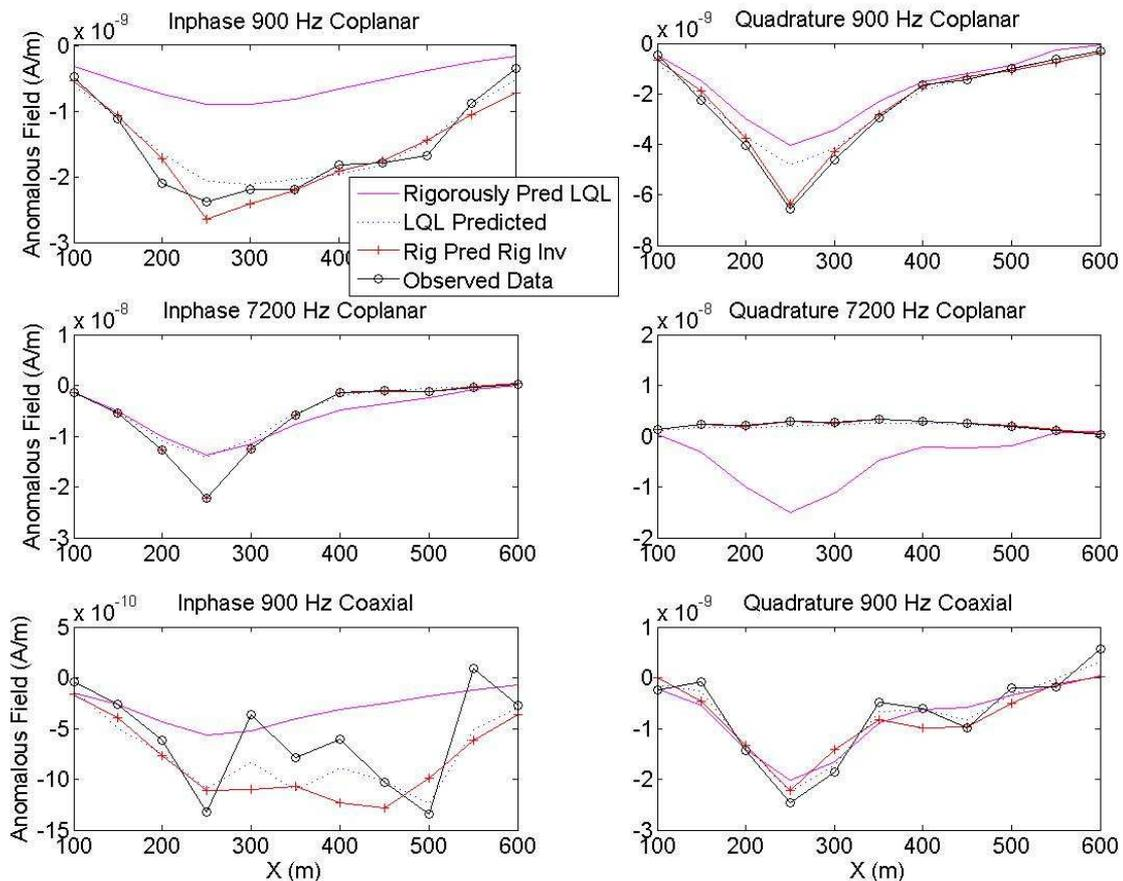
Figure 3: Predicted and observed data for a synthetic AEM survey. The data shown are along a profile at  $y=300$  m. The curve "Rigorously Pred LQL" corresponds to the rigorously predicted data for the LQL solution. "LQL Predicted" curve is the approximately predicted data to the LQL solution. The line marked as "Rig Pred Rig Inv" shows the final predicted data. Also shown are the synthetic data. Note the large error introduced into the observed data of the coaxial channel using 1.5 ppm error.
