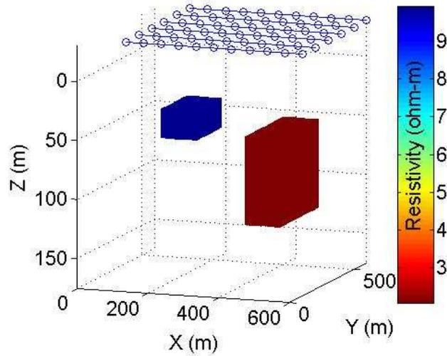
Figure 1: The geoelectric model with two conductive bodies and AEM survey design. The upper body is 10 ohm-m, and the lower body is 2 ohm-m. They are imbedded in a 100 ohm-m halfspace. The flight lines are shown as blue lines with circles for sounding locations.
