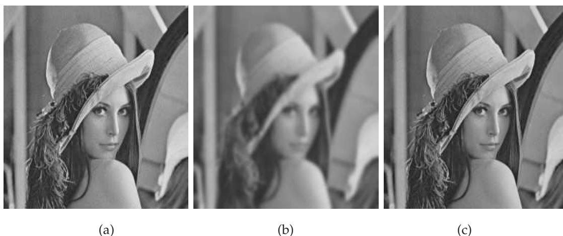
Figure 2: Deblurring using the backward isotropic diffusion equation, left: original image, middle: blurred image, right: recovered image.
