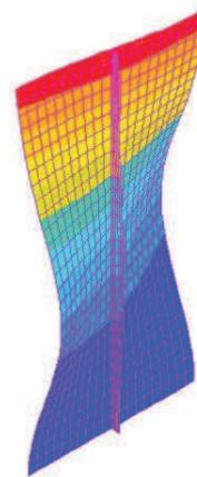
Figure 7: The third buckling mode of the structure.
