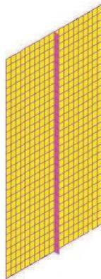
Figure 4: The finite element model of the structure: two panels and one stringer.
