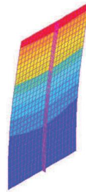
Figure 5: The first buckling mode of the structure.
