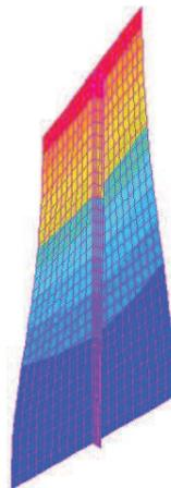
Figure 6: The second buckling mode of the structure.
