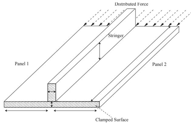
Figure 3: Description of the finite element based test: the solid arrows are the uncertain variables.
