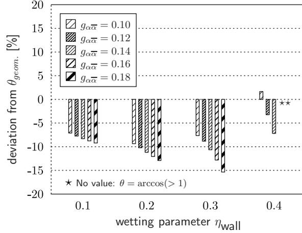
Figure 7: Deviation (in percent) of the contact angle measured using the approach of Huang et al. from geometrical measurements. The initial volume of the droplet is  $70^3 l.u.^3$ .
