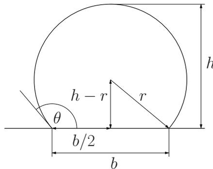
Figure 2: Geometrical measurement of the contact angle. The contact angle can be determined by measuring the diameter of the base  $b$  and the height  $h$ . The radius of the droplet is given by  $r = (4h^2 + b^2)/8h$ .
