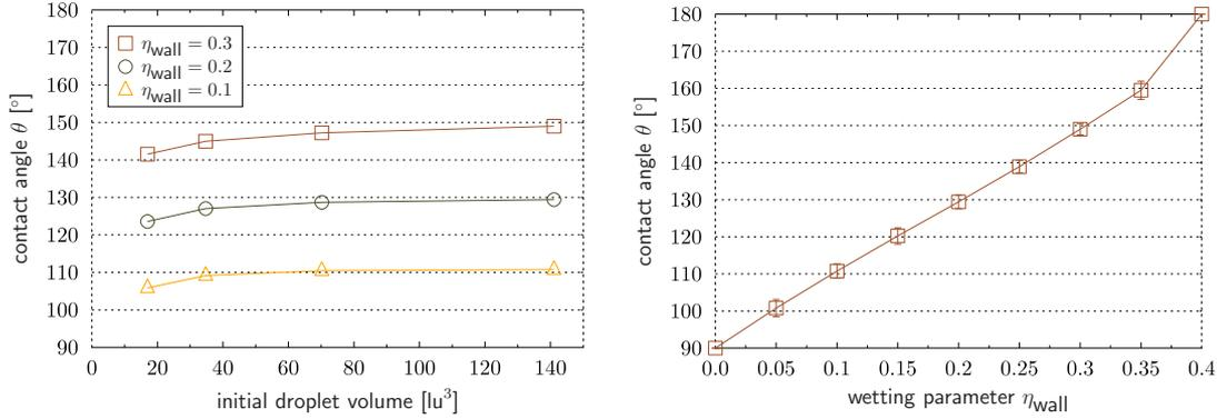
Figure 4: Left: dependence of  $\theta$  on the droplet size for different fluid-surface interactions.  $g_{\alpha\bar{\alpha}}$  is kept fixed at 0.16. Right: contact angle versus wetting parameter  $\eta_{\text{wall}}$  for a droplet with initial volume  $141^3$  and  $g_{\alpha\bar{\alpha}} = 0.16$ . The error bars denote values obtained from assuming the interface position being given by half the maximum absolute value of the order parameter  $\phi$ . Lines drawn are a guide to the eye.
