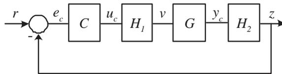
FIG. 2. A constrained feedback system
