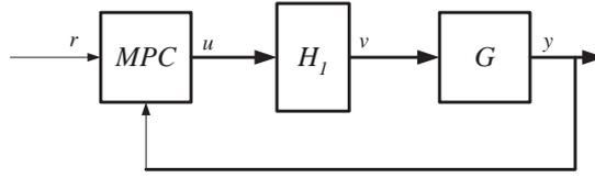
FIG. 3. Networked-based MPC control system
