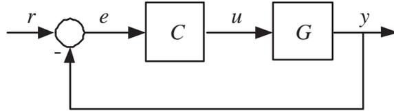
FIG. 1. A typical feedback system
