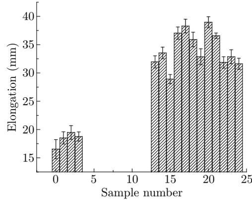
Fig. 5: The elongation of PTT filaments after creep test under different heat-setting conditions.
