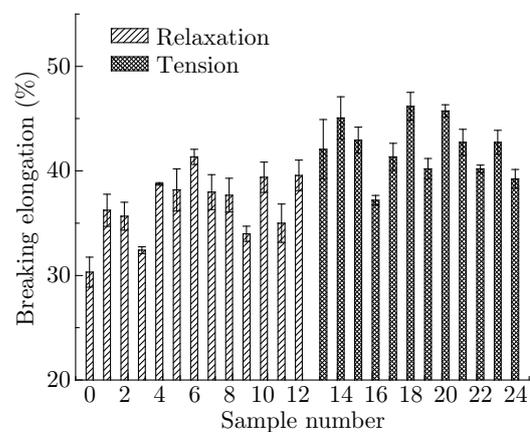
Fig. 2: The breaking elongation of PTT filaments under different heat-setting conditions.
