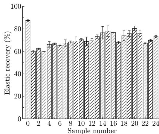
Fig. 4: The elastic recovery of PTT filaments under different heat-setting condition.
