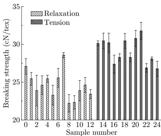
Fig. 1: The breaking strength of PTT filaments under different heat-setting conditions.
