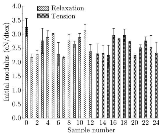
Fig. 3: Young's modulus of PTT filaments under different heat-setting conditions.
