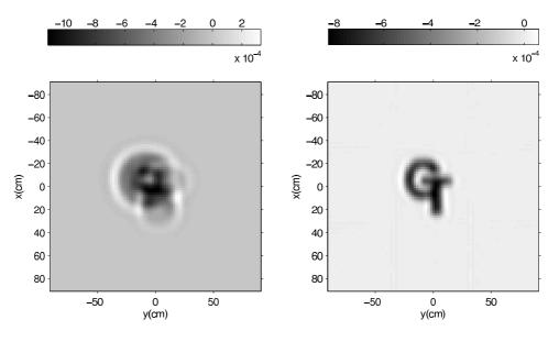
Figure 5: The horizontal slice of the raw image and the 3-D migration reconstructed image of the GT plywood in free space. Left: The GPR raw data. Right: 3-D NUFFT migrated data at the plywood surface. The estimated size is 38 cm wide, 44 cm high and 1.76 cm thick.
