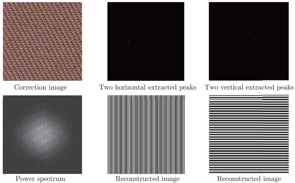
Fig. 3: The reconstructed images of twill woven fabric
