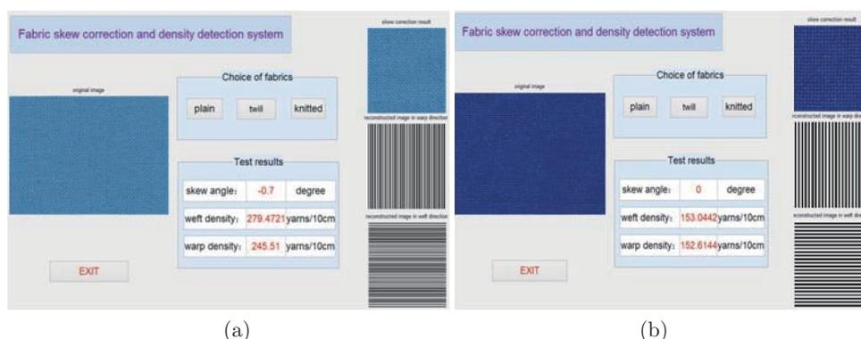
Fig. 7: Fabric skew correction and density detection system: (a) Test result of plain woven fabric; (b) Test result of knitted fabric
