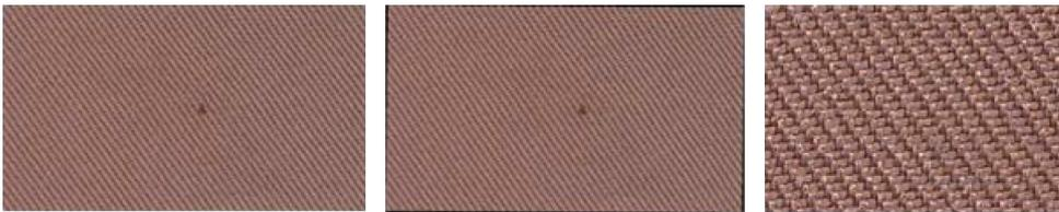
Fig. 4: The skew correction results of twill woven fabrics
