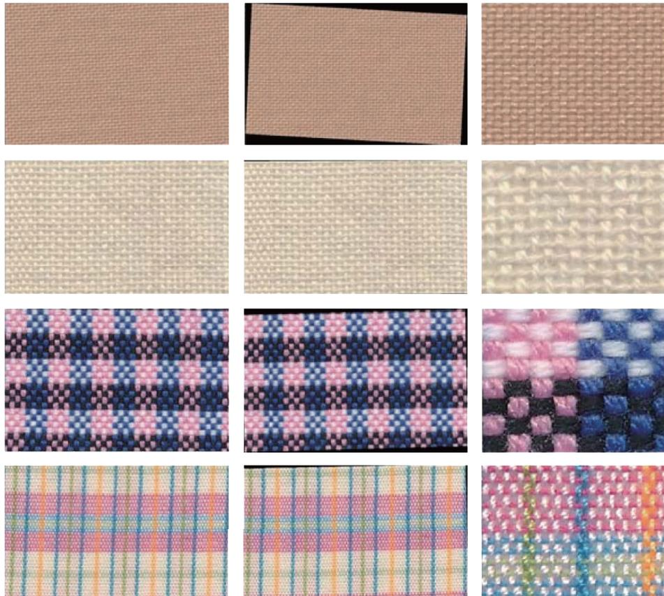
Fig. 6: The skew correction results of plain woven fabrics
