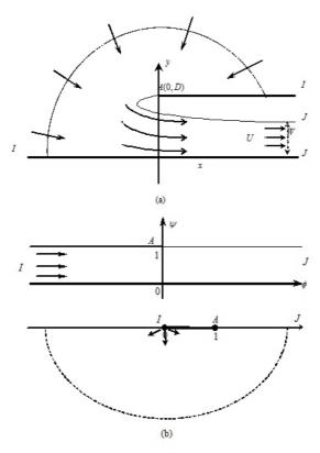
Figure 2: Sketch of the two-dimensional flow entering a slit (a) in physical z-plane, (b) in f and  $\zeta$ -planes.
