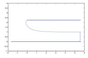
Figure 4: The profile of free surface flow for F = 2.5, producing contraction coefficient 0.445.
