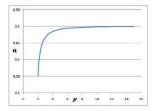
Figure 5: Plot of the contraction coefficient  $\alpha$  versus Froude number F.
