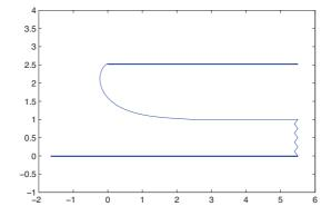
Figure 3: The profile of free surface flow for F = 2.1, producing contraction coefficient 0.396.
