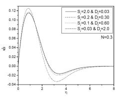
Figure 7: Microrotation profiles for various values of  $S_r$  and  $D_f$ .
