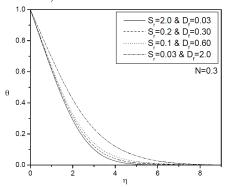
Figure 8: Temperature profiles for various values of  $\mathcal{S}_r$  and  $\mathcal{D}_f.$
