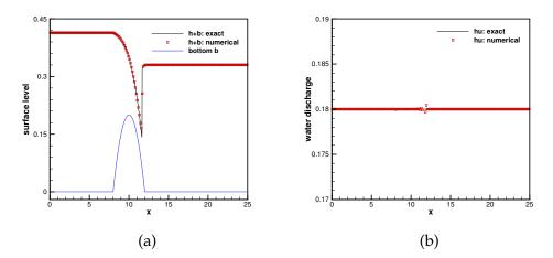
Figure 5: Free surface level h+b (a) and water discharge hu (b) of the Case B in Section 4.1.5 at t=200s.
