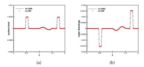
Figure 2: Free surface level h+b (a) and water discharge hu (b) of the small pulse example in Section 4.1.3 at t=0.2s.
