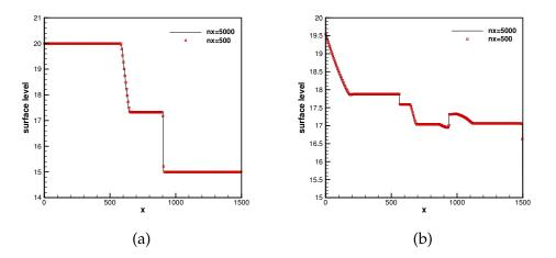
Figure 3: Free surface level h+b of the example in Section 4.1.4 at t=15s (a) and t=60s (b).
