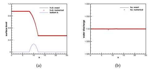
Figure 4: Free surface level h+b (a) and water discharge hu (b) of the Case A in Section 4.1.5 at t=200s.
