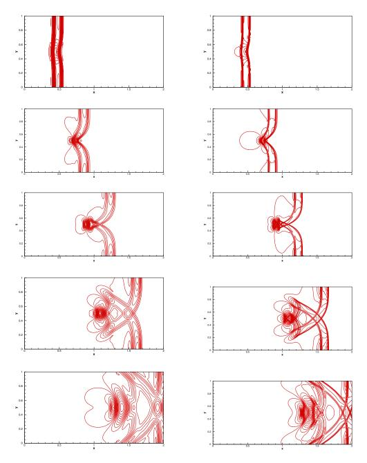
Figure 8: Thirty contours of free surface level h+b of the example in Section 4.2.2. From top to bottom: at t=0.12 s from 0.99942 m to 1.00656 m; at t=0.24 s from 0.99318 m to 1.01659 m; at t=0.36 s from 0.98814 m to 1.01161 m; at t=0.48 s from 0.99023 m to 1.00508 m; and at t=0.6 s from 0.99514 m to 1.00629 m. Left:  $200 \times 100$  cells. Right:  $600 \times 300$  cells.
