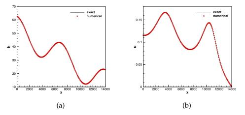
Figure 7: Water depth h (a) and flow velocity u (b) of the example in Section 4.1.6 at t=7552.13s.
