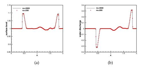
Figure 1: Free surface level h+b (a) and water discharge hu (b) of the big pulse example in Section 4.1.3 at t=0.2s.
