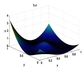
Figure 5: Example 4.7: The numerical solution of the local  $P^4$ -DG method at t = 1.
