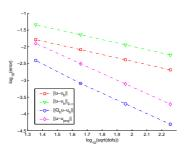
Figure 7: Convergence orders of  $u - u_h$ ,  $Q_h u - u_h$  and  $u - \hat{u}$  in different norms (piecewise constant).
