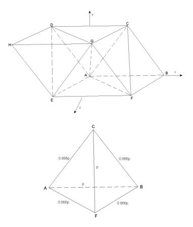
Figure 4: The Par6 assembly and the tetrahedron in Par6
