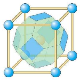
Figure 2: Basic Voronoi cell of BCC configuration.
