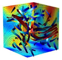
FIGURE 1. The velocity solution to the Ethier-Steinman problem with a = 1.25, d = 1 at t = 0 on the  $(-1, 1)^3$  domain. The complex flow structure is seen in the streamribbons in the box and the velocity streamlines and speed contours on the sides.
