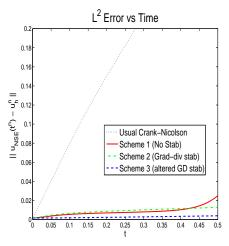
FIGURE 2. The plot above shows  $L_2$  error of the velocity vs time for the four schemes of test 2. We see in the plot that the stabilizations add accuracy to the enhanced-physics scheme, and that the altered grad-div stabilization gives slightly better results than the usual grad-div stabilization. It can also be seen that the enhanced-physics scheme is far more accurate in this metric than the usual Crank-Nicolson scheme.
