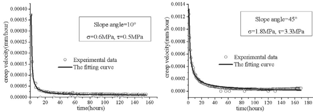
Figure 5: The fitting curves of creep velocity of structural planes.
