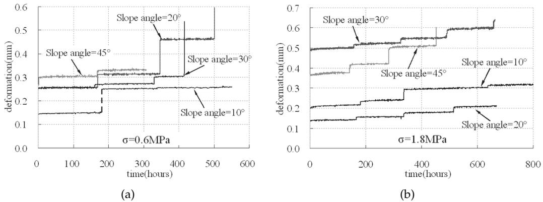
Figure 2: The curves of shear creep test process of structural planes with different slope angles.
