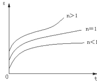
Figure 7: Creep curves of modified Burger model.
