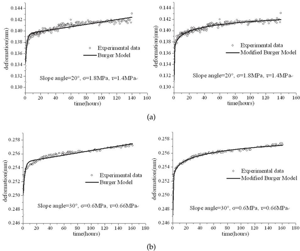
Figure 8: The test curves fitting graph of the modified Burger model and Burger model.
