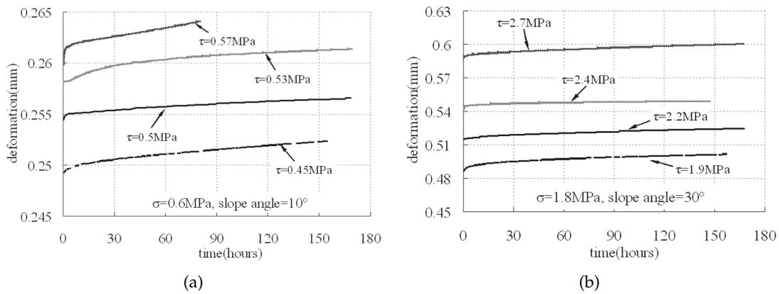
Figure 3: The grading curves of shear creep of 10° and 30° structural planes.
