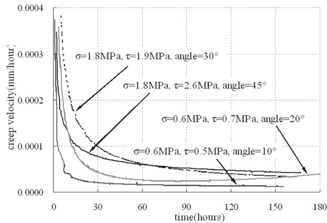
Figure 4: The creep velocity curves of structural planes with different slope angles.
