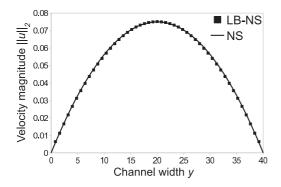
Figure 6: Parabolic profile measured in the middle of a  $40\!\times\!40$  channel. The continuous line corresponds to the Navier-Stokes solution whereas the black squares represent the hybrid Lattice Boltzmann–Navier-Stokes solution. Another parabolic curve was obtained from a pure Lattice Boltzmann simulation, which is close to identical to both the Navier-Stokes and the Lattice Boltzmann–Navier-Stokes profile and therefore has been left out in this figure.
