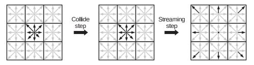
Figure 1: The Lattice Boltzmann algorithm for the D2Q9 model. In the collide step, the post-collision distributions  $f_i^*(x,t) = f_i(x,t) + \Delta_i(f - f^{eq})$  are computed locally in each cell. In the streaming step, the distribution functions are moved along their respective lattice velocities  $c_i$  to their neighbours, i.e.  $f_i(x+c_idt,t+dt) = f_i^*(x,t)$ .
