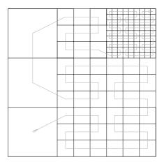
Figure 2: Example of a 2D discrete Peano curve on a corresponding adaptive Cartesian grid.
