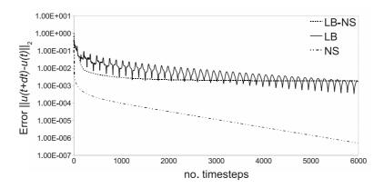
Figure 8: Error  $\|u(t+dt)-u(t)\|_2$  measured over time for the channel scenario. The continuous line represents the pure Lattice Boltzmann solution, the dash-dotted line describes the error decay for the Navier-Stokes solver. The dashed curve corresponds to the coupled Lattice Boltzmann–Navier-Stokes solution.
