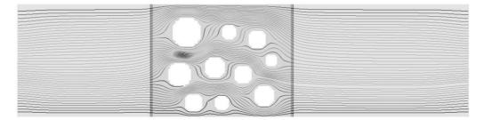
Figure 9: Application of the hybrid Navier-Stokes–Lattice Boltzmann scheme to a two-dimensional directed flow through a simplified porous medium represented by randomly placed spheres. The two vertical dark-grey lines represent the boundaries between the two outer Navier-Stokes domains and the Lattice Boltzmann domain which contains the porous medium.
