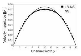
Figure 7: Parabolic profile measured in the middle of a  $20\!\times\!20$  channel. The continuous line corresponds to the Navier-Stokes solution whereas the black squares represent the hybrid Lattice Boltzmann–Navier-Stokes solution.
