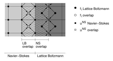
Figure 5: Overlap grid for coupled simulations. The velocities  $u^{NS}$  need to be computed from the neighbouring Lattice Boltzmann cells, the particle distribution functions  $f_i$  have to be constructed from the velocity and pressure values of the corresponding Navier-Stokes cells.
