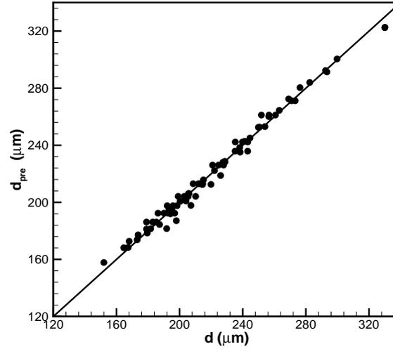
Figure 15: Comparison of droplet diameter between the fitting results  $d_{pre}$  from Eq. (4.3) and the simulation results  $d$ .
