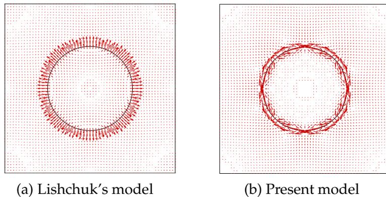
Figure 3: Comparison of the spurious velocities of a droplet in stationary fluid with  $\sigma=0.01$  and  $R=30\delta_x$  for (a) the model proposed by Lishchuk et al. [42] with the magnification rate of 1:  $1.5 \times 10^5$  and (b) the present model with the magnification rate of 1:  $1.5 \times 10^7$ .
