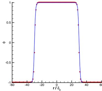
Figure 2: The profile of order parameter along the cross section of a droplet with  $R=30\delta_x$ . The discrete symbols represent the simulation results of the present LB model and the solid line is the theoretical profile given by Eq. (3.2).
