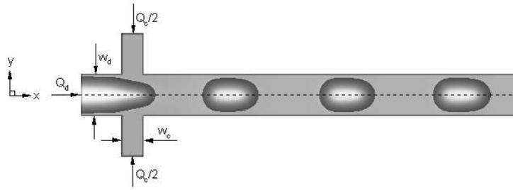
Figure 7: The schematic diagram of droplet formation in a cross-junction microchannel, where  $w_d$ ,  $w_c$  are the widths of the main and lateral channels, and  $Q_c$  and  $Q_d$  are the inlet volumetric flow rates of the continuous and dispersed phases.
