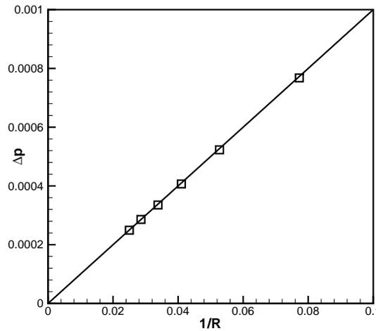
Figure 1: Comparison of the LBM results ( $\square$ ) with the Laplace's law (the solid line) for pressure jump across a stationary droplet interface.
