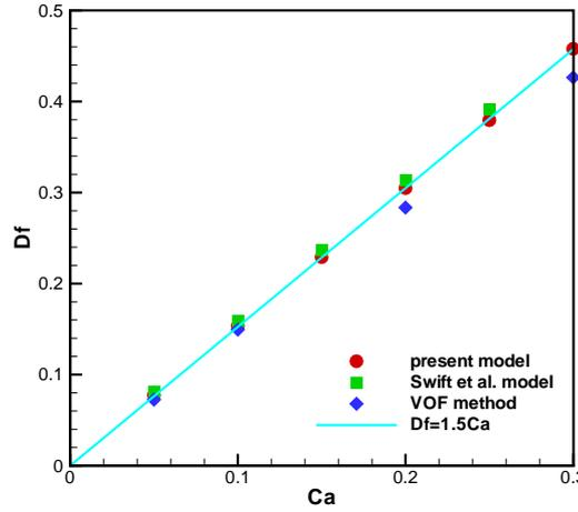
Figure 4: Taylor deformation parameter  $Df$  as a function of the capillary number.
