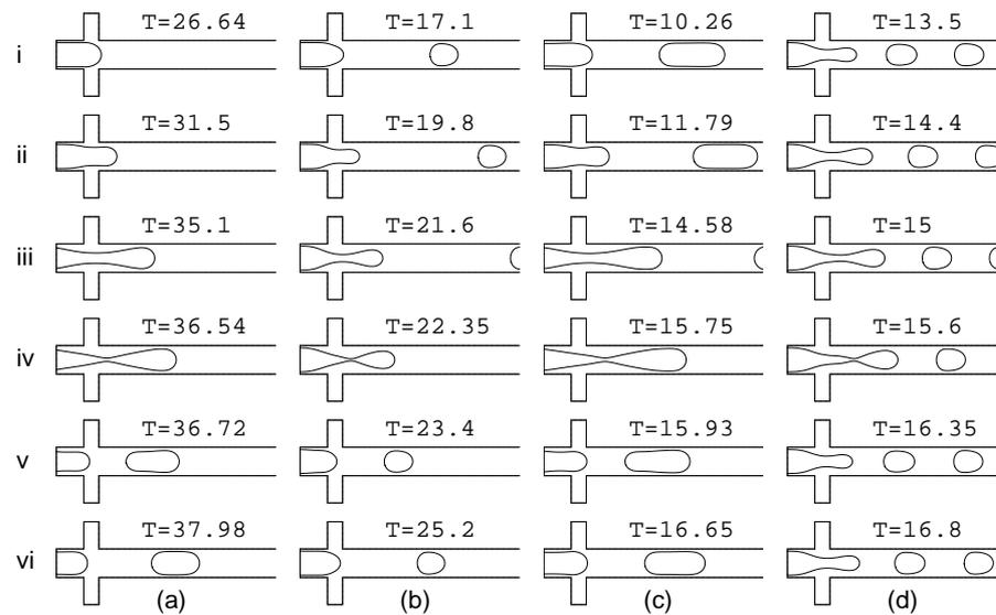
Figure 12: A series of instantaneous states of droplet formation for (a)  $Q=1/6$ ,  $Ca=0.0024$ ; (b)  $Q=1/6$ ,  $Ca=0.024$ ; (c)  $Q=1/2$ ,  $Ca=0.0024$  and (d)  $Q=1/2$ ,  $Ca=0.024$ . The viscosity ratio  $\lambda=1/4$ , and the dimensionless time is defined as  $T=u_{ct}/w_c$ .
