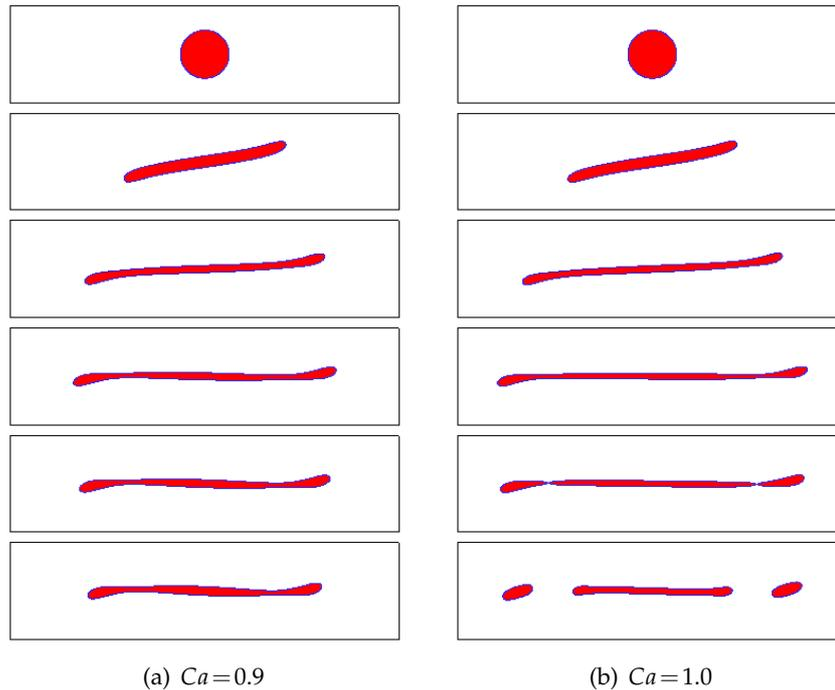
Figure 6: Snapshots of the droplet evolution under simple shear flow at  $\lambda=1$ ,  $Re=1.0$  for (a)  $Ca=0.9$  and (b)  $Ca=1.0$ , taken at times  $T=\{0,6,12,24,27,30\}$ .
