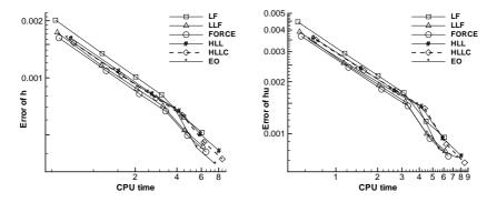
Fig. 3.4. Dam break on a flat bed. The  $L_1$  numerical error and the CPU time (unit: second) using the log scale for h (left) and hu (right) by the WENO methods based on different fluxes on meshes with N = 200, 300, 400, 500, 600, 700 cells.
