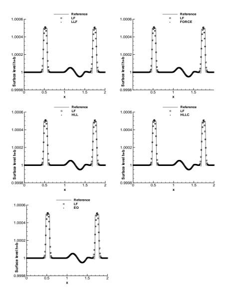
Fig. 3.9. Pulse over a hump. The surface level h + b. Solid lines: the reference solution; hollow square: the results computed by the WENO-LF scheme; plus symbols: the results computed by the WENO-LLF (top left), WENO-FORCE (top right), WENO-HLL (middle left), WENO-HLLC (middle right), and WENO-EO (bottom).
