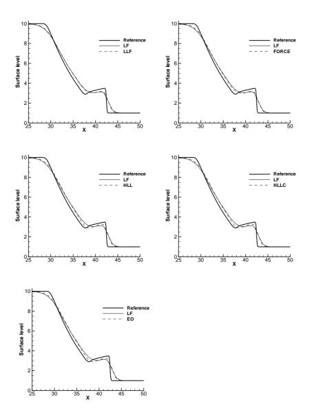
Fig. 3.12. Trans-critical break of a circular dam at t = 0.69s. The surface level distributing along the line y = 25 from x = 25 to x = 50. Heavy solid lines: the reference solution; Solid lines: the results computed by the WENO-LF scheme; Dashed line: the results computed by the WENO-LLF (top left), WENO-FORCE (top right), WENO-HLL (middle left), WENO-HLLC (middle right), and WENO-EO (bottom).
