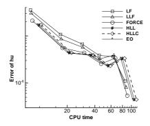
Fig. 3.6. Steady trans-critical flow over a hump without a shock. The  $L_1$  numerical error (left) and the  $L_{\infty}$  numerical error for hu and the CPU time (unit: second) using the log scale by the WENO methods based on different numerical fluxes on meshes with N = 200, 300, 400, 500, 600, 700 cells.
