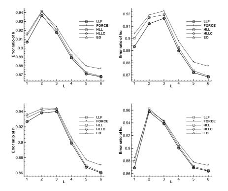
Fig. 3.1. An accuracy test over a sinusoidal hump. Error ratio of the  $L_1$  numerical error for h (top left) and hu (top right) and of the  $L_{\infty}$  numerical error for h (bottom left) and hu (bottom right) by the WENO methods based on different fluxes to that by the WENO-LF method on meshes with  $N = 25 \cdot 2^{L-1}$ , (L = 1, 2, ...6) cells.
