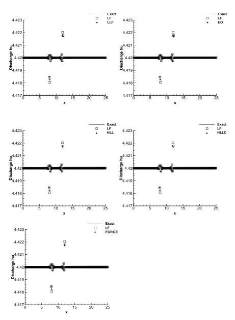
Fig. 3.7. Steady sub-critical flow over a hump. The discharge *hu*. Solid lines: the exact solution; hollow square: the results computed by the WENO-LF scheme; plus symbols: results computed by the WENO-LLF (top left), WENO-EO (top right), WENO-HLL (middle left), WENO-HLLC (middle right), and WENO-FORCE (bottom).
