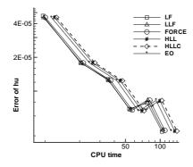
Fig. 3.8. Steady sub-critical flow over a hump. The  $L_1$  numerical error for hu and the CPU time (unit: second) using the log scale by the WENO methods based on different numerical fluxes on meshes with N = 200, 300, 400, 500, 600, 700 cells.
