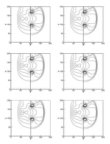
Fig. 3.11. Asymmetric break of a dam. Surface level contours at time t = 7.2s. 15 contours between 4 and 9.5. The WENO-LF (top left), WENO-LLF (top right), WENO-FORCE (middle left), WENO-HLL (middle right), WENO-HLLC (bottom left), and WENO-EO (bottom right).
