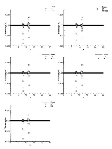
Fig. 3.5. Steady trans-critical flow over a hump without a shock. The discharge *hu*. Solid lines: the exact solution; hollow square: the results computed by the WENO-LF scheme; plus symbols: results computed by the WENO-LLF (top left), WENO-FORCE (top right), WENO-HLL (middle left), WENO-HLLC (middle right), and WENO-EO (bottom).
