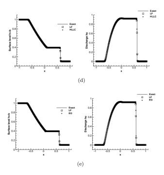
Fig. 3.3. Dam break on a flat bed at t = 0.1s. Left: the surface level h+b; Right: the discharge hu. Solid lines: the exact solution; hollow square: the results computed by the WENO-LF scheme; plus symbols: results computed by the (a)WENO-LLF, (b)WENO-FORCE, (c)WENO-HLL, (d)WENO-HLLC, and (e)WENO-EO.
