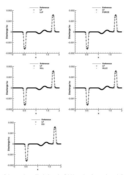
Fig. 3.10. Pulse over a hump. The discharge *hu*. Solid lines: the reference solution; hollow square: the results computed by the WENO-LF scheme; plus symbols: the results computed by the WENO-LLF (top left), WENO-FORCE (top right), WENO-HLL (middle left), WENO-HLLC (middle right), and WENO-EO (bottom).
