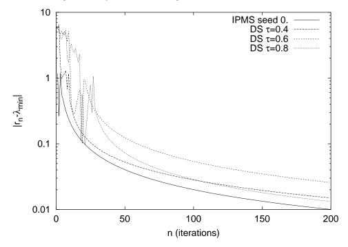
Figure 7: Comparison of  $|r(\vec{x}_n) - \lambda_{\min}|$  versus number of iterations n for matrix  $M_2$  with the Inverse Power Method and the dynamical system with three different values of  $\tau$ .
