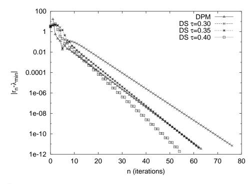
Figure 4: Comparison of  $|r(\vec{x}_n) - \lambda_{\max}|$  versus number of iterations n for matrix  $M_1$  with the Power Method and the dynamical system with three different values of  $\tau$ .
