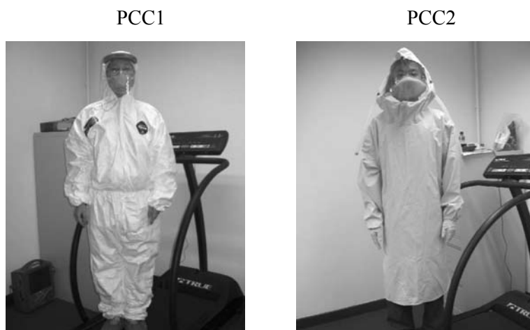
Figure 1 Two different types of personal protective clothing ensembles used in wear experiment
