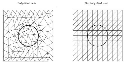
Fig. 1.1. The body-fitted and non-body-fitted mesh in 2D.
