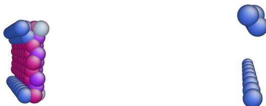
Figure 14: Atomic configuration of state B. Left: irregular atoms; Right: atoms with coordinate number 13.
