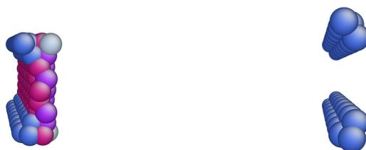
Figure 15: Atomic configuration of state C. Left: irregular atoms; Right: atoms with coordinate number 13.
