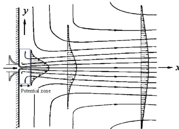
Figure 14: The laminar 2D free jet flow.
