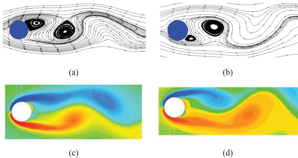
Figure 20: Plot of streamlines (a, b) and vorticity (c, d) at two times for  $Re=100$ .
