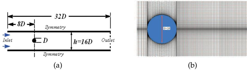
Figure 17: Flow configuration for simulation of flow past a cylinder placed symmetrically in a planar channel and (b) mesh grids around circular cylinder.
