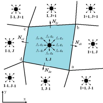
Figure 1: Schematic of the FV discretization with cell-centered lattice.
