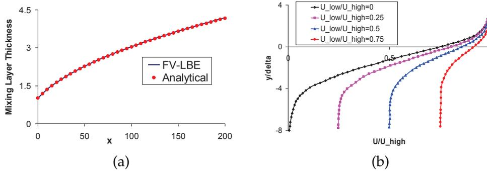
Figure 12: (a) Streamwise growth of the vorticity at  $Re=300$ . Curve fit using  $\delta_w = 0.2875\sqrt{x+12.371}$  and (b) Velocity profiles for the mixing layers at different velocities.
