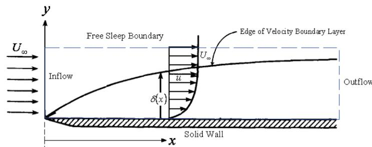
Figure 7: Sketch of boundary layer on a flat plate.
