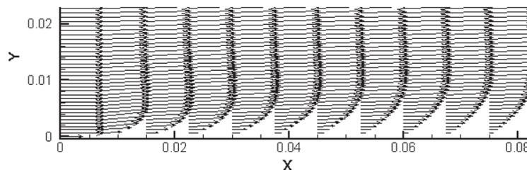
Figure 8: Velocity vectors of boundary layer flow at  $Re = 25$ .
