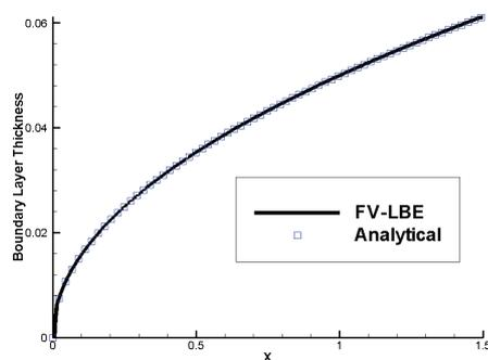
Figure 10: Growth of the boundary layer thickness.
