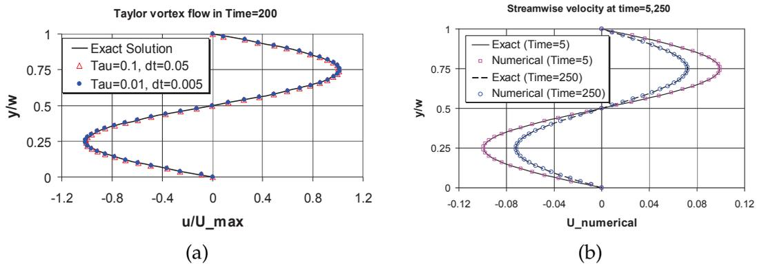
Figure 5: Analytical and calculated streamwise velocity profiles for the Taylor-Vortex flow simulation for  $\tau = 0.1, 0.01$  and time  $t = 5, 250$ .
