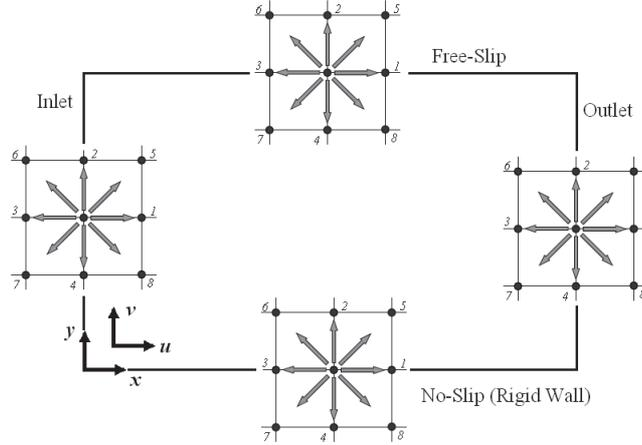
Figure 2: Physical boundaries of the solution domain and lattice model on typical boundaries.
