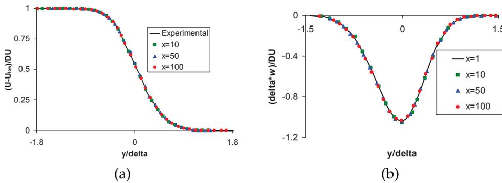
Figure 13: The cross-stream variation of the normalized (a)  $u$ -component velocity, (b) vorticity.
