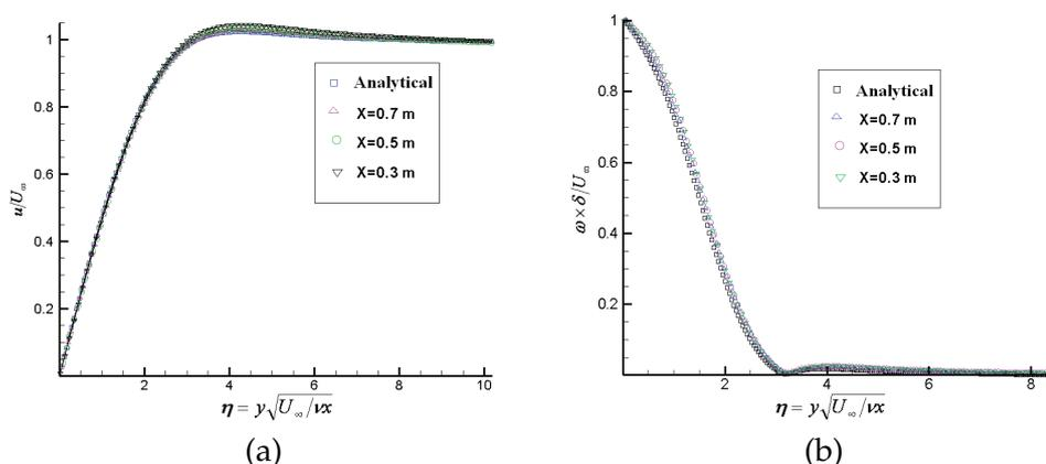
Figure 9: (a) Velocity and (b) vorticity distribution in the boundary layer along a flat plate.
