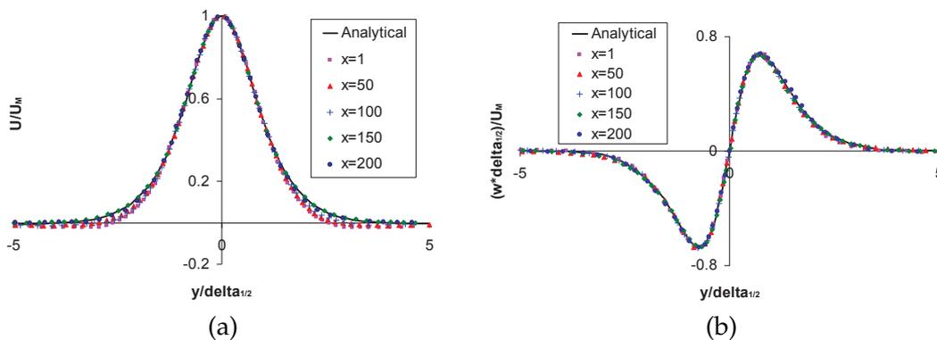
Figure 16: The cross-stream variation of the normalized (a)  $u$ -component velocity, (b) vorticity.
