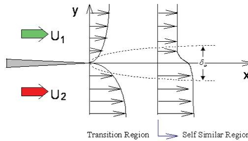
Figure 11: Schematic of plane mixing layer.
