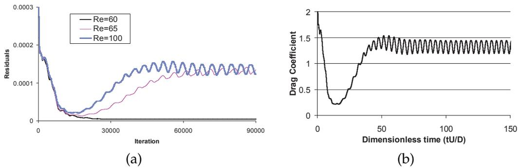
Figure 19: (a) Behavior of velocities residuals at  $Re=60$ , 65 and 100 and (b) variation of drag coefficient with time at  $Re=100$ .
