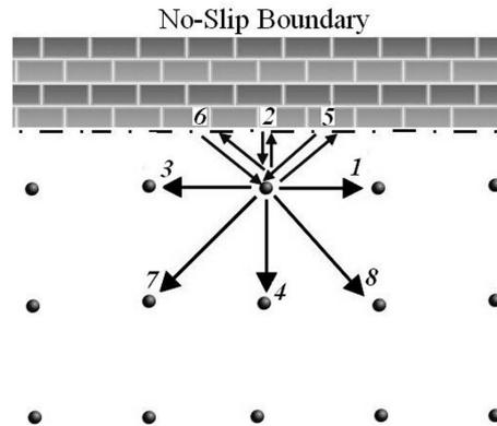
Figure 3: Schematic of bounce-back algorithm for straight wall.
