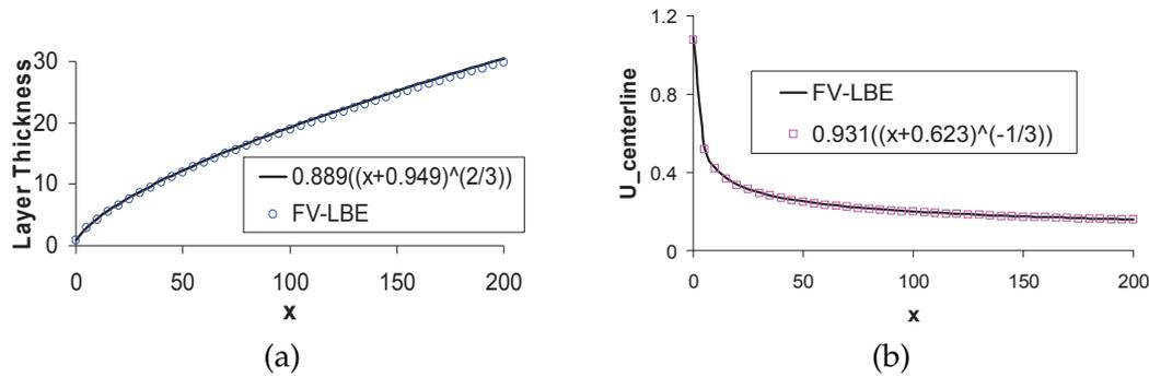
Figure 15: (a) Growth of the jet half-width, (b) decay of the centerline velocity of free jet.
