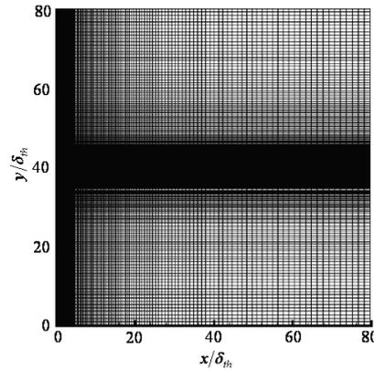
Figure 6: Used geometry in the jet/mixing layer flow simulation.
