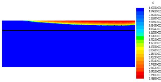
Figure 9: Concentration in the case of  $C_{in} = 14 \text{ mol/m}^3, u_{in} = 3 \text{ m/s}, I = 1.5 \text{ A cm}^{-2}$ .
