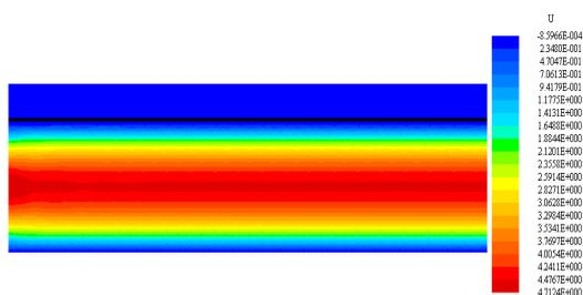
Figure 6: Horizontal two-phase mixture velocity in the case of  $C_{in} = 14 \text{ mol/m}^3$ ,  $u_{in} = 3 \text{ m/s}$ ,  $I = 1.5 \text{ Acm}^{-2}$ .
