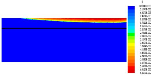
Figure 11: Liquid water saturation in the case of  $C_{in} = 14 \text{ mol/m}^3, u_{in} = 3 \text{ m/s}, I = 1.5 \text{ A cm}^{-2}$ . The evaporation front separating the two-phase zone from the single-phase region is approximately represented by  $s = 0.01$ .
