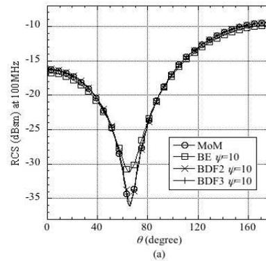
Figure 3: The RCS with oversampling factor  $\psi=5$  and  $\psi=10$  for the sphere as a function of elevation angle.
