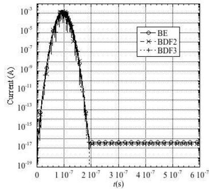
Figure 2: The average surface current by BE, BDF2 and BDF3 with stabilization. Note that the y-axis differs from that Fig. 1 to accommodate the undershoot of BDF3.
