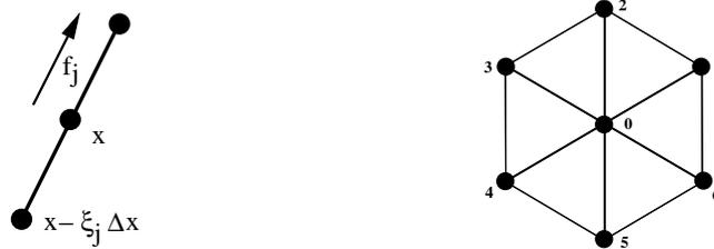
Figure 1: Typical stencil of a lattice Boltzmann scheme for a Bravais lattice (left) ; both opposite directions  $\xi_j$  and  $-\xi_j$  connect two vertices of the mesh. Local numbering of the six neighbours (right) of the D2T7 lattice Boltzmann scheme on triangles.
