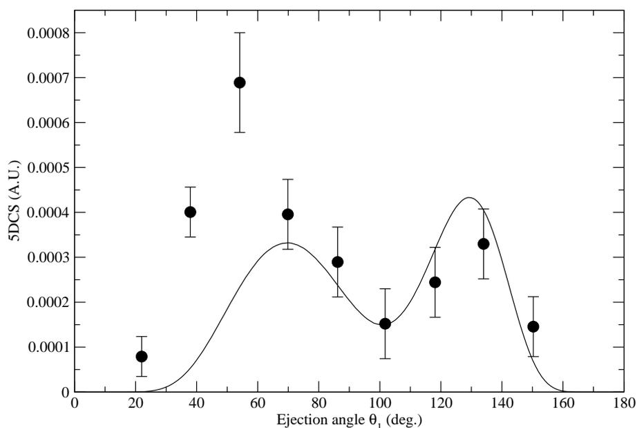
Figure 5: 5DCS for the double ionization in coplanar geometry of molecular hydrogen (solid line: theoretical results) and helium targets (full circles: experimental data), in the *symmetric geometry* mode; both ejected electrons emerge with symmetric angles with respect to the incident beam direction, i.e.,  $\theta_1 = -\theta_2$ .
