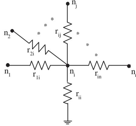
Figure 1: The resistance network of node  $n_i$ .
