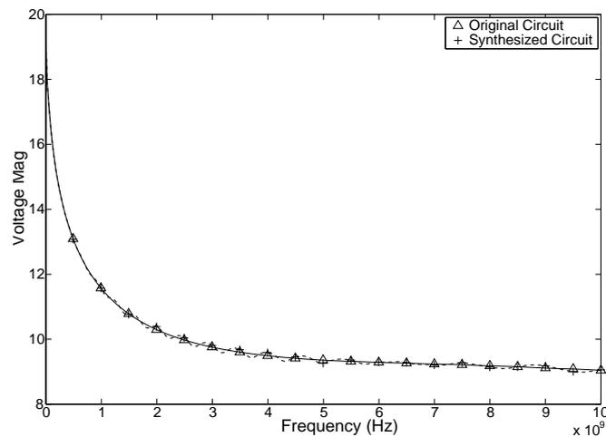
Figure 8: Comparison of AC simulation results of RCS circuit and the synthesized RLC circuit with  $tol = 10^{-8}$ .
