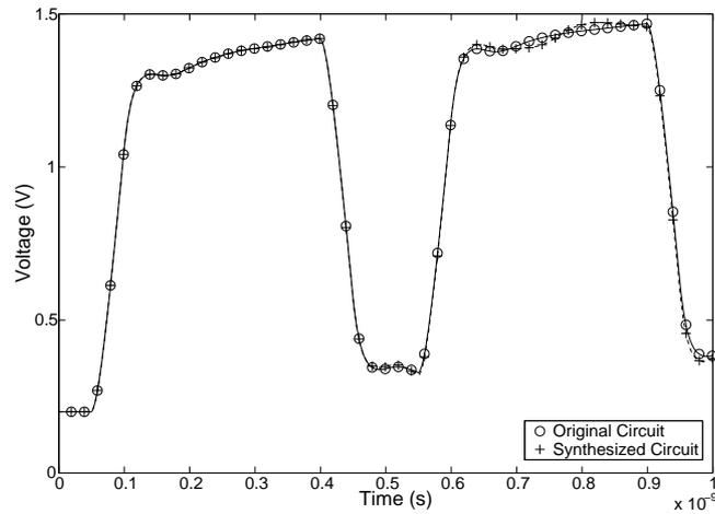
Figure 10: Comparison of transient simulation results of RLC circuit and the synthesized RLC circuit with  $tol = 10^{-8}$ .
