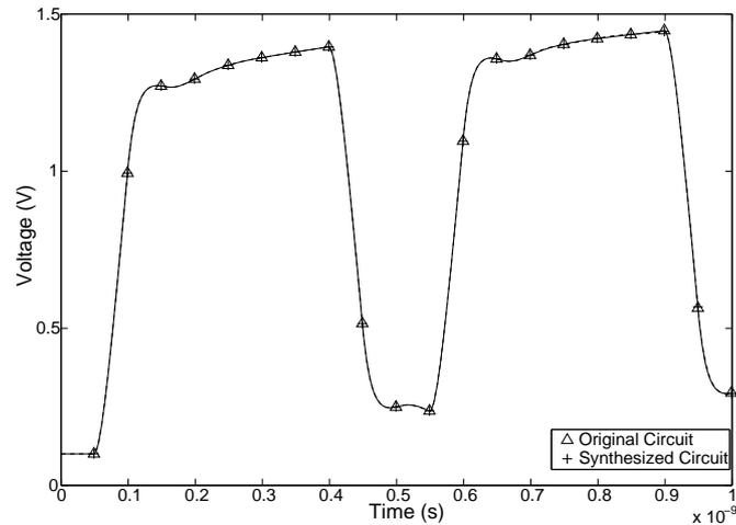
Figure 7: Comparison of transient simulation results of RCS circuit and the synthesized RLC circuit with  $tol = 10^{-8}$ .
