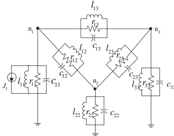
Figure 2: A sample circuit with 3 nodes synthesized by unstamping.
