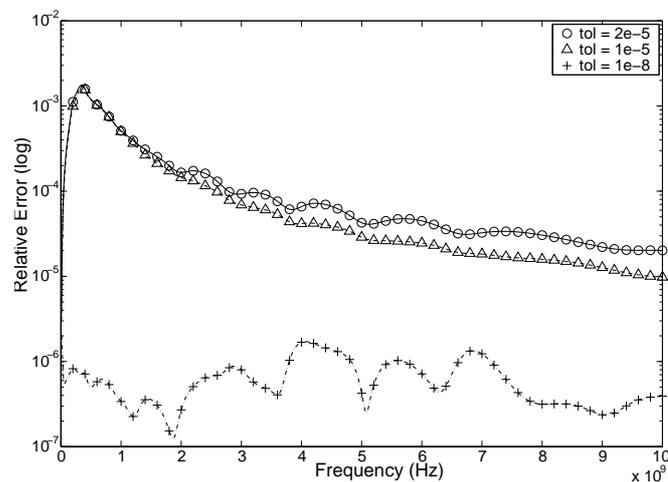
Figure 9: Error induced by diagonalization and regularization with different  $tol$  values of the RLC example.
