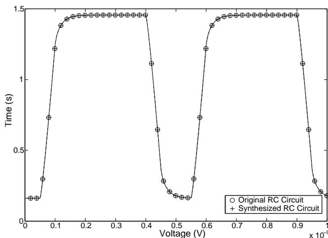
Figure 4: Comparison of transient simulation results of the original RC circuit and the synthesized RC circuit.
