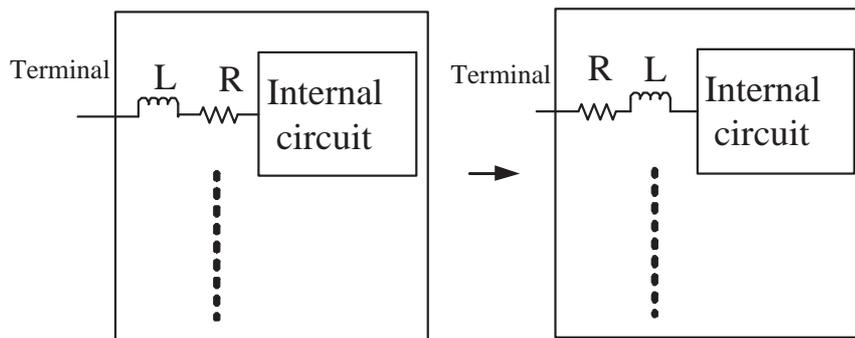
Figure 3: Swapping the positions of R and L elements doesn't change the input-output transfer characterization of the interconnect circuit.
