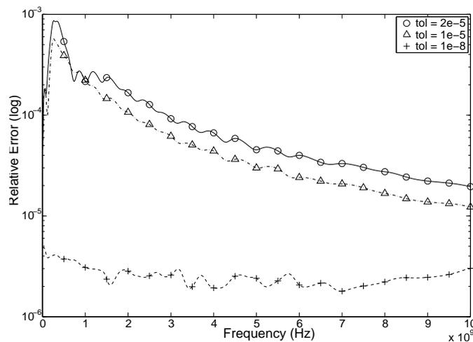
Figure 6: Error induced by regularization with different  $tol$  values of the RCS example.
