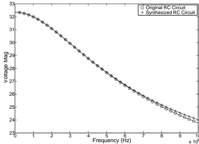
Figure 5: Comparison of AC simulation results of the original RC circuit and the synthesized RC circuit.
