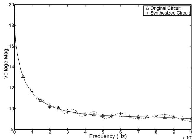
Figure 11: Comparison of AC simulation results of RLC circuit and the synthesized RLC circuit with  $tol = 10^{-8}$ .
