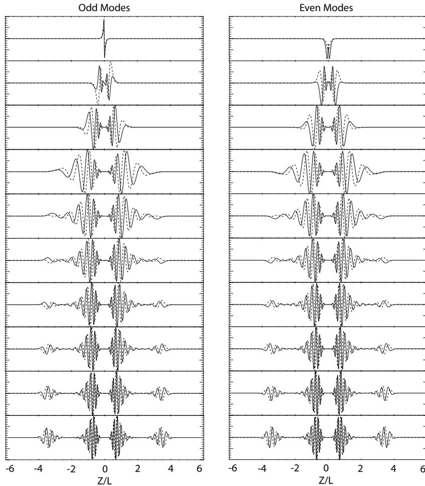
Figure 1: Mode structures associated with the lower-hybrid drift instabilities, where the electric potential  $\phi$  are plotted versus  $z/L$ , solid curves represent the real part of  $\phi$ , and the dotted curves stand for the imaginary part of  $\phi$ . Modes with node number 1,7,13, $\dots$ ,55 are selected as samples for odd-symmetrical eigenfunctions, and modes with node number 0,6,12, $\dots$ ,54 for even-symmetrical.
