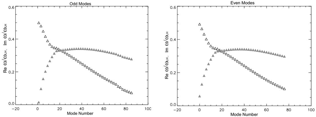
Figure 2: Real ( $\Delta$ ) and imaginary ( $\blacktriangle$ ) parts of the eigenvalues,  $\text{Re}\omega/\omega_{LH}$  and  $\text{Im}\omega/\omega_{LH}$ , corresponding to the solutions shown in Fig. 2, versus the mode number:  $1,3,5,\dots$ , for odd modes, and  $0,2,4,\dots$ , for even modes.
