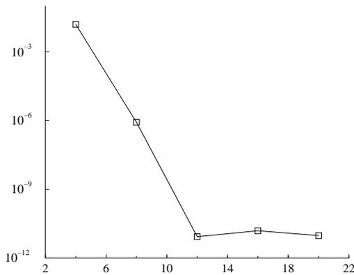
Figure 2:  $L^2$  error norm  $\|\mathbf{u} - \mathbf{u}_N\|_{(L^2(\Omega))^2}$  as a function of the polynomial degree on the rectangle domain.
