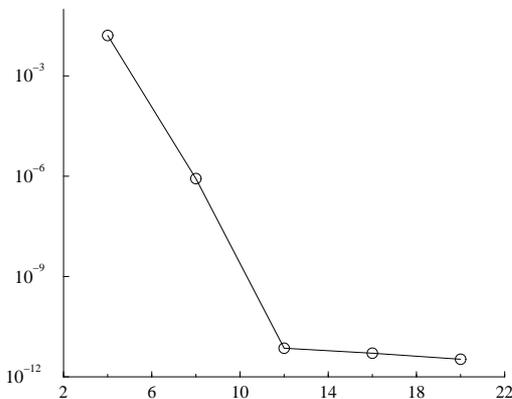
Figure 4:  $L^2$  error norm  $\|\mathbf{u} - \mathbf{u}_N\|_{(L^2(\Omega))^2}$  as a function of the polynomial degree  $N$  on the L-shaped domain.
