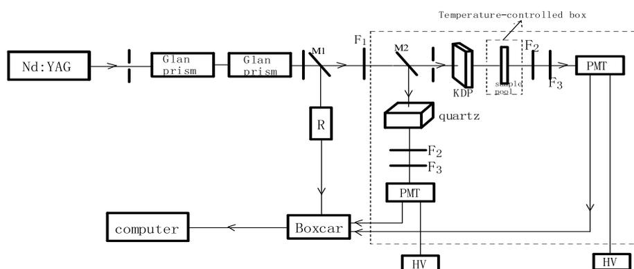
Figure 2: Schematic diagram of all optical poling.
