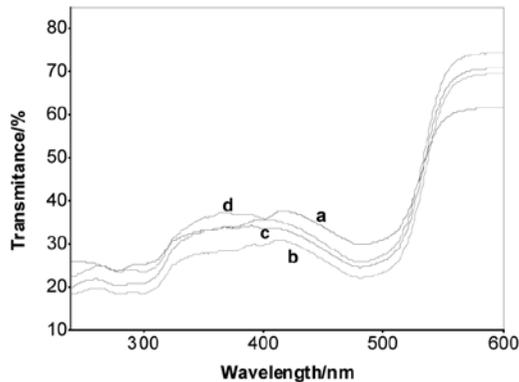
Figure 3 Spectrogram of adding different content of adhesive (a) 0% adhesive, (b) 0.2% adhesive, (c) 0.8% adhesive, (d) 1.5% adhesive
