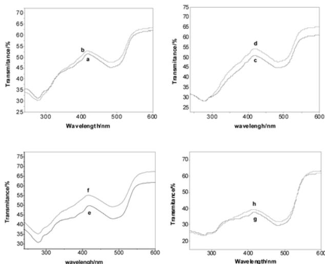
Figure 2 Spectrogram of the fabric after treated with different content of TiO<sub>2</sub> (a) 0.2%, (b) sample a after 50 washing circles, (c) 0.5%, (d) sample c after 50 washing circles, (e) 0.8%, (f) sample e after 50 washing circles, (g) 1.5%, (h) sample g after 50 washing circles
