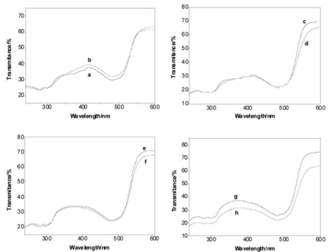
Figure 4 Spectrogram of the fabric treated with different content adhesive (a) 0.0 %; (b) sample a after 50 washing circles; (c) 0.2% adhesive; (d) sample c after 50 washing circles; (e) 0.8% adhesive; (f) sample e after 50 washing circles; (g) 1.5% adhesive; (h) sample g after 50 washing circles
