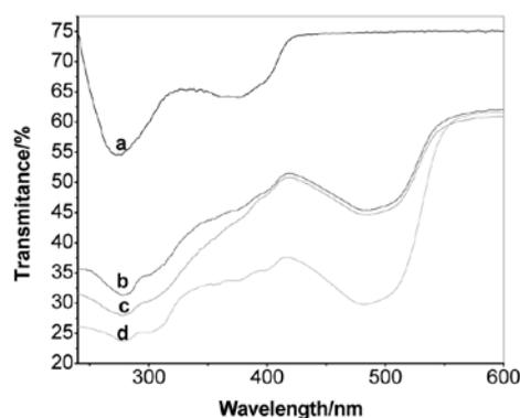
Figure 1 Spectrogram diagram of cotton fabrics treated with different content of nano-TiO<sub>2</sub> (a) grey cloth, (b) 0.2 % nano-TiO<sub>2</sub>, (c) 0.5 % nano-TiO<sub>2</sub>, (d) 1.5 % nano-TiO<sub>2</sub>
